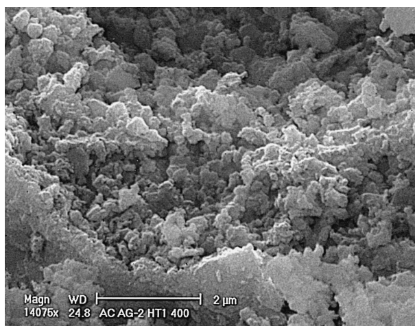
Fig. 5. SEM micrograph of \text{LiCoO}_2 obtained by heat treating the precursors to 400^\circ\text{C} for 2 h. Note the presence of agglomerated clusters of particles whose primary particles are in the range of \approx 70 nm.
